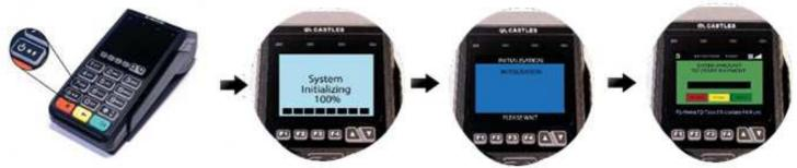
Press and hold the power button (above the red key) until the screen lights up. The terminal will power on and initialise for use.
