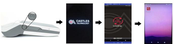
Press and hold the power button (on the left side of the terminal) until the screen lights up. The terminal will power on and initialise for use.
